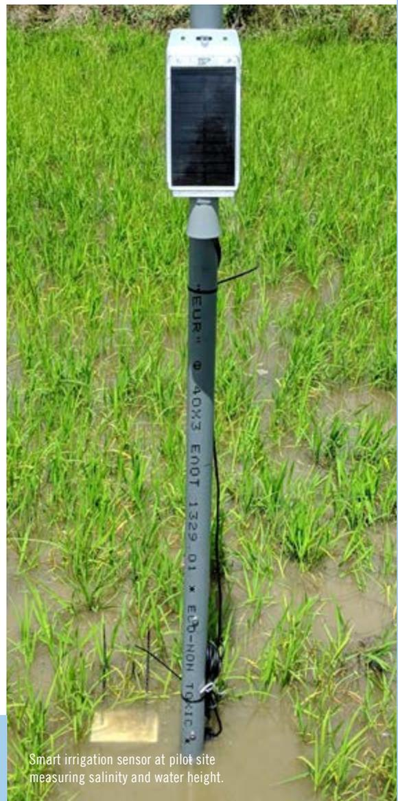
Smart irrigation sensor at pilot site measuring salinity and water height.
